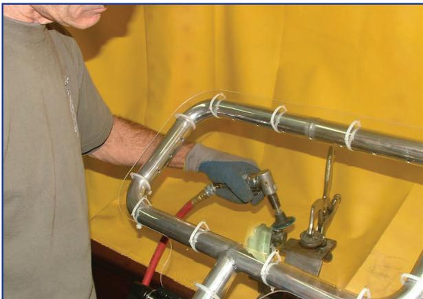
The effective low pressure area formed in front of the AirShield is shallow. This prevents the shield from causing turbulence when used along with a HEPA ventilation unit. Turbulence would tend to increase the production of airborne particulates. The Lancs AirShield is designed to work as a standalone unit for low kinetic energy work such as table top inspections and valve maintenance, or in combination with other controls for surface destructive work.
